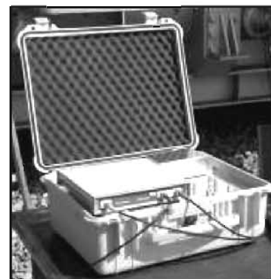
Figure 36: FRA measurement with OMICRON FRAnalyzer
